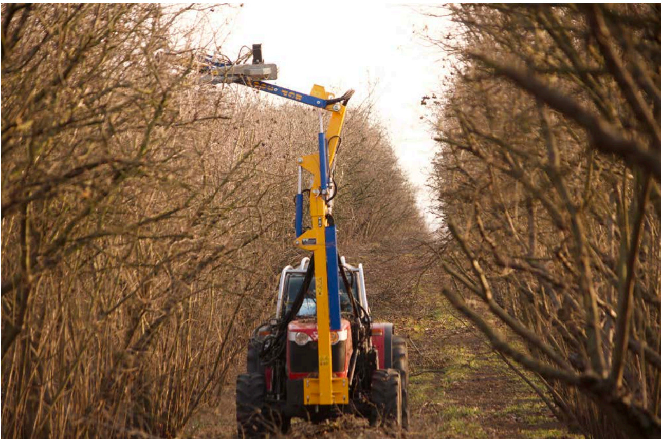
Figure 7 - Mechanical hedger during "topping" application in a mature hazelnut orchard.
