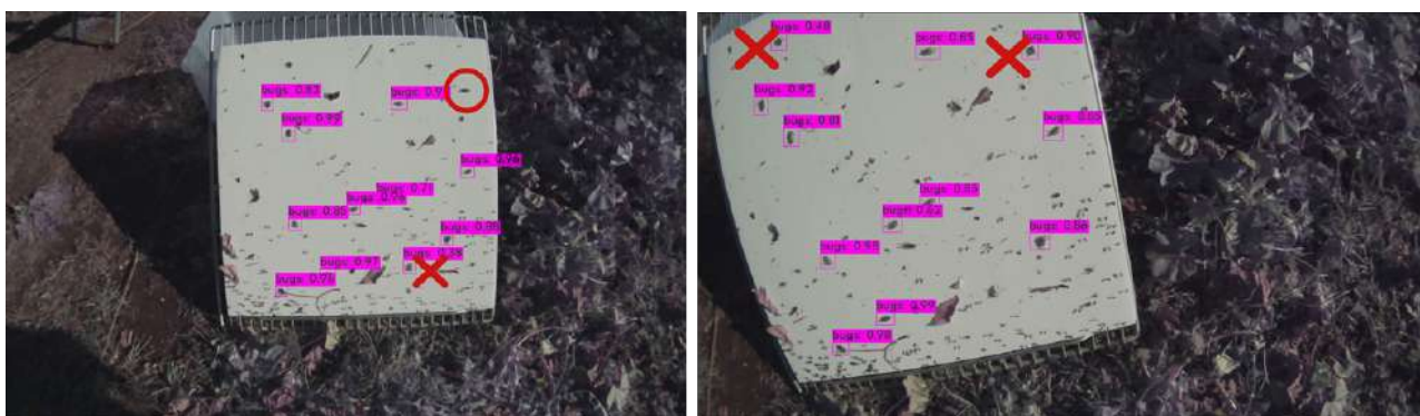
Figure 7 Examples of predicted bounding boxes with respective confidence scores. The false positives are highlighted with red x-marks and the only false negative with a red circle.
